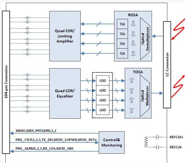
**Figure 1. CFP2 LR4 Optical Transceiver functional block diagram**
